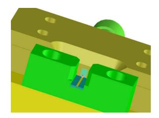
After the Transition is rotated back by three degrees, the RF pin should make contact in the middle of the microstrip.
