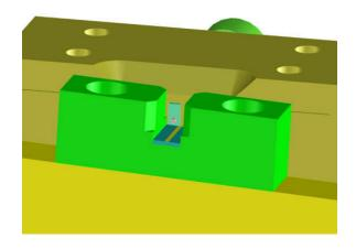
This picture shows the position of the RF pin when the Transition is tilted by three degrees. When attaching the first screw, make certain that the RF pin is in this position.
