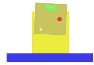
When attaching the Transition to a calibration standard, insert the upper screw first and tilt the transition by approximately three degrees. Insert the screw all the way, but do not tighten it. This maneuver protects the RF pin while mounting the Transition.
