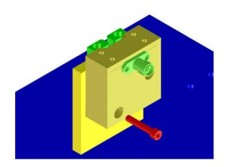
Carefully rotate the Transition back to the horizontal position, and insert the second screw. The weight of the Transition will automatically apply sufficient force for the RF pin to make contact. Tighten screw number one and number two securely.
