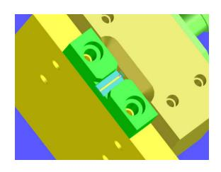
Re-check the RF pin, and make certain that it is properly seated on the microstrip. It should be exactly in the middle of the microstrip line.
